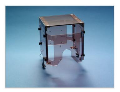
The X-ray indicator with markers is used to impose fiducials on X-ray image of the patient to be used for target localization during treatment planning.
