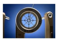
Cross-Hairs Kit in Stainless Steel is used with Leksell Stereotactic System® to intraoperatively check the placement of inserted electrodes, catheters or other instruments in relation to the set target point. Cross-Hairs Kit is used with Leksell Stereotactic System® to intraoperatively check the placement of inserted electrodes, catheters or other instruments in relation to the set target point.
