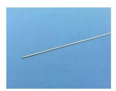
Universal Guide tube for MicroMacro or Micro Electrode and Medtronic DBS lead. The guide tube is fixated in the MicroGun and is not moving with the electrode when advanced towards the target. The inner guide tube for the MicroMacro or Micro Electrodes ends 10 mm before target and the outer guide tube for the Medtronic DBS lead ends 13 mm before target. Inner guide tube Outer Diameter = 1.40 mm, Inner Diameter = 1.0 mm, Length = 206 mm.
