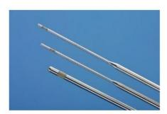
One Monopolar Brain Lesion Electrode for stimulation, impedance measurement and lesioning. Tip diameter = 1 mm and tip length = 2 mm. Outer diameter 2.2 mm.
