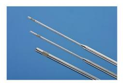
One Monopolar Brain Lesion Electrode for stimulation, impedance measurement and lesioning. Tip diameter = 1.5 mm, tip length 2 mm and outer diameter 2.2 mm.
