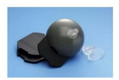
The Radiation Phantom with Cassettes is used for calibrating the absorbed dose rate of Leksell Gamma Knife®. Radiation Phantom with Cassettes The phantom is divided into two halfe spheres between which a cassette can be inserted. The cassettes allow film dosimetry, TLD and dose measurment by means of a small ionization chamber. The cassettes are made of polystyrene and are 10 mm thick.
